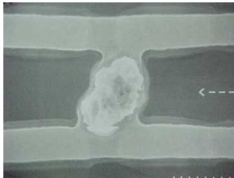
Photo 2-4 Dust-induced Wiring Short
