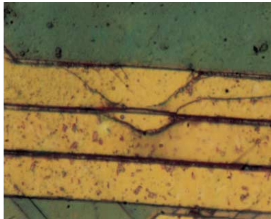
Photo 2-7 Cracking due to Al Sliding
