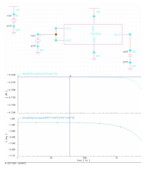
The input applied has a DC bias voltage of 2V with an ac magnitude of 1V. The graphs shows AC gain for common mode input, the differential gain is 56dB. So CMRR will be
